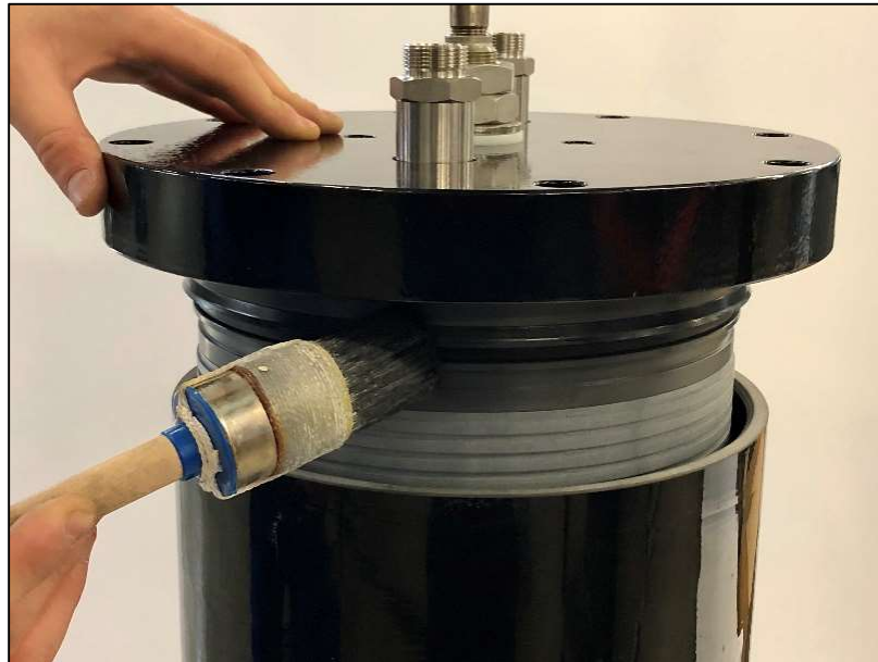
Figure 26. Top pressure plate lip seal lubrication
