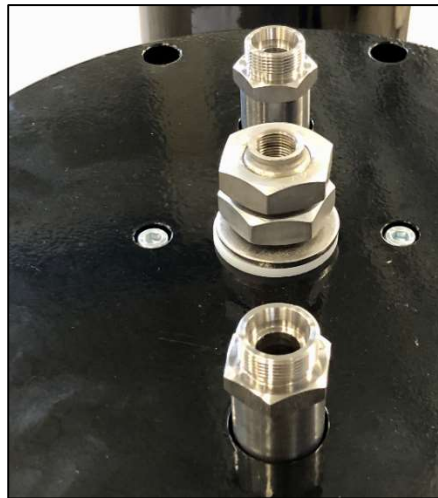
Figure 21. Top plates assembly second nut installation
