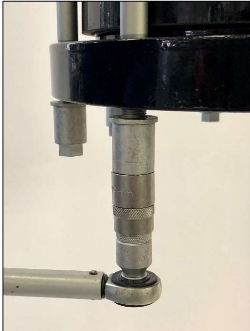
Figure 30. Bottom washers and cap nuts installation
