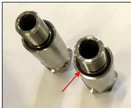
Figure 16. Feed and concentrate adaptors O-rings installation
