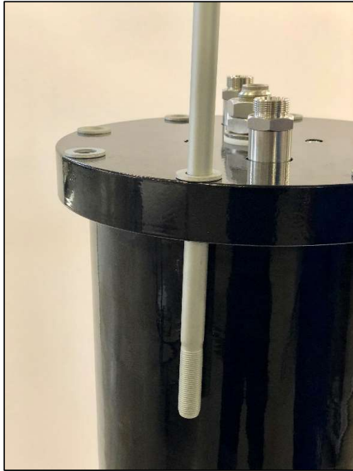
Figure 29. Tension rods insertion
