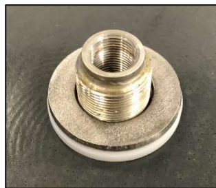
Figure 19. Top plates assembly washers positioning
