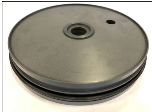
Figure 14. Top pressure plate lip seal installation
