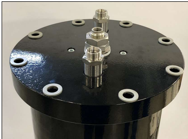
Figure 28. Tension rods top washers placement
