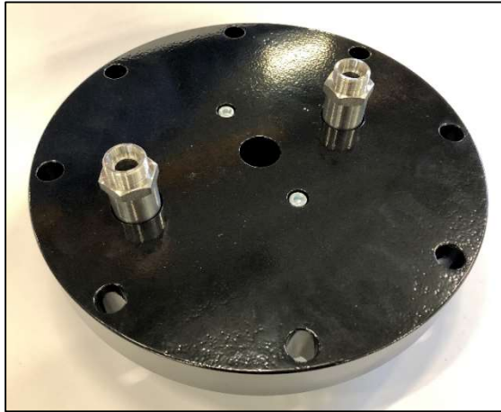
Figure 17. Feed and concentrate adaptors installation
