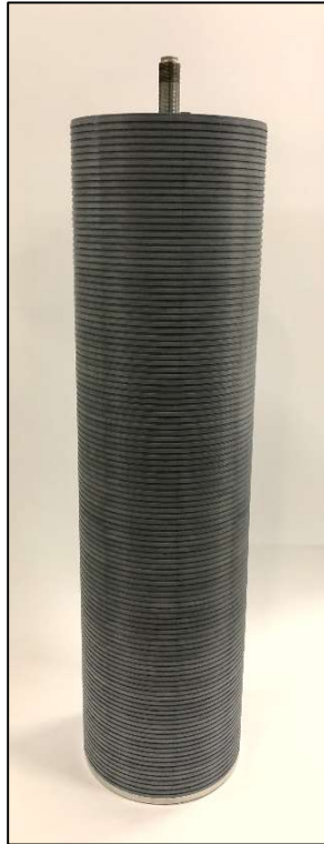
Figure 12. Support plates stacking onto the permeate anchor
