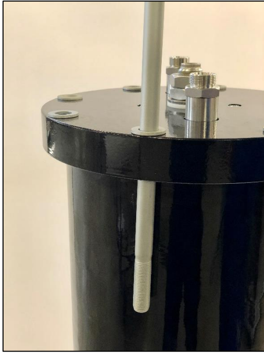
Figure 29. Tension rods insertion
