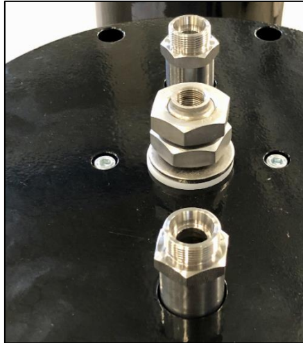
Figure 21. Top plates assembly second nut installation
