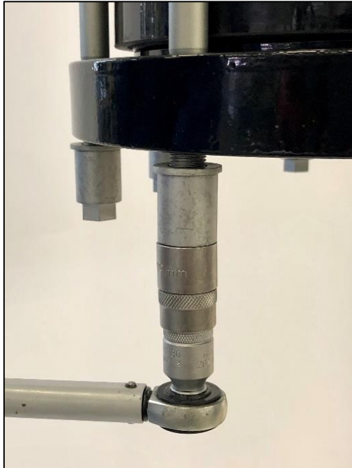
Figure 30. Bottom washers and cap nuts installation
