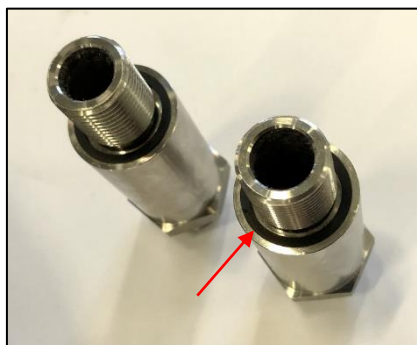
Figure 16. Feed and concentrate adaptors O-rings installation
