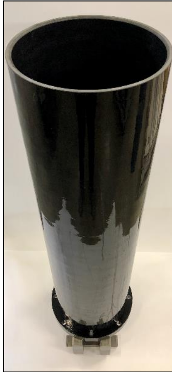
Figure 24. Pressure vessel fitting onto the bottom plates assembly
