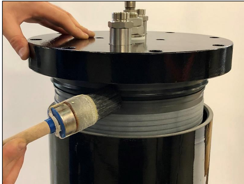
Figure 26. Top pressure plate lip seal lubrication
